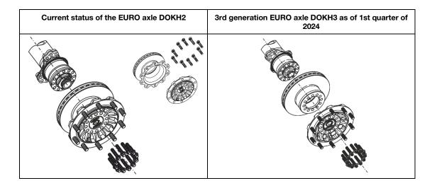
• The axle nut with left-hand/right-hand thread and with a slit for clamping on the axle stub for securing, was replaced by a standard axle nut with flange and right-hand thread on both sides.
