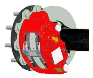
The approved gigant EuroAchse (DOKH2 09010 4345H1) will be extended by the at the moment lightest brake caliper Haldex DBT 19LT for the standard program.
