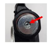
The grease emerges at a defined point through a pressure relief opening.
