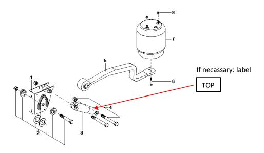
Orientated shock absorbers are marked with a label "TOP" on the shock absorber body of the lower fixing point. The label "TOP" has to be orientated upwards to ensure a proper function of the shock absorber.
