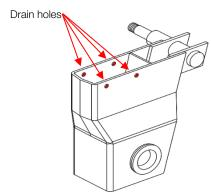
Air suspension bracket with drain holes starting in the
