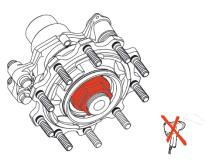
4. Put on the retainer bolt by hand and tighten with the torque wrench to the correct tightening torque
