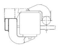
The centre axle lift (CAL-C) is supported on the C-profile's crossbeam by the welded bellows support. The lift boom is welded on the axle body. An air bellows that is installed between the bellows support and lift boom is used to push up the axle
