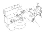
The Twinlift is supported only on the air suspension bracket. The Twinlift support is welded onto the air suspension bracket according to the specifications in the drawing. Due to the clamp, the Twinlift FB100 can only be mounted on the single
