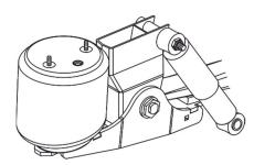
The side axle lift (SAL) is supported on the chassis' longitudinal beam. The pivot point is the spring fitting on the air suspension bracket. The SAL can be installed on the left or right side.
