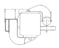
The centre axle lift (CAL-C) is supported on the C-profile's crossbeam by the welded bellows support. The lift boom is welded on the axle body. An air bellows that is installed between the bellows support and lift boom is used to push up the axle.
