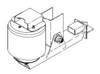
The centre axle lift (CAL) is supported on the chassis' crossbeam. The pivot point is on the suspension bracket. The console is welded on the axle body.
