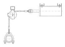
A cable is used to pull up the axle via deflection rollers. A pneumatic cylinder is used as the pulling device. This special version is used whenever there are severe space-related problems.
